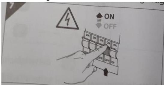
4. Reinsert the fuse or switch on the circuit breaker at the fuse box (I-position) (see **fig.7**).
