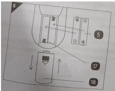
[17] Battery compartment [18] Battery compartment cover
