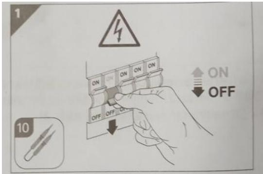
1. Make sure that there is no voltage on the ceiling cable to which the product is to be connected. To do this, remove the fuse or switch off the circuit breaker in the fuse box (0 position).
