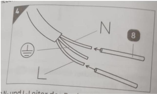
1. Push the N and L conductors of the ceiling cable of the domestic installation through the protective conduits [8] (see **fig.4**).
