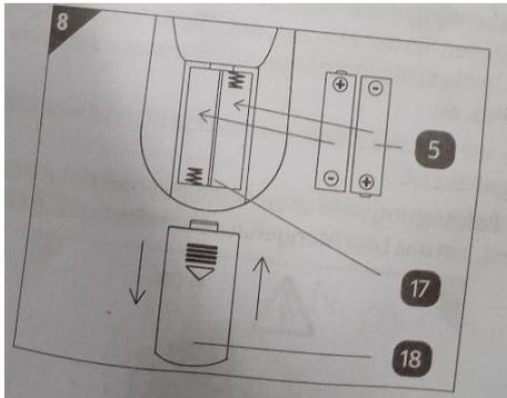
[17] Battery compartment [18] Battery compartment cover
